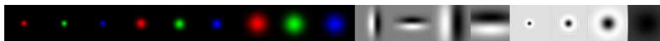
Figure 2.3: Illustration of texton filters. Note that the filters operate in CIELab color space (RGB shown for illustrative purposes only).
